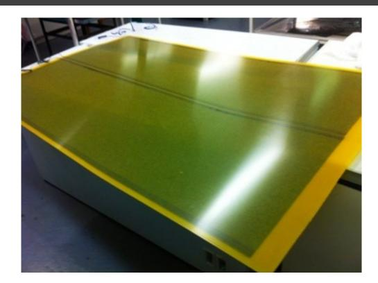
LH **PowerFilm** is embedded in a woven glass fiber fabric impregnated with a tooling style quality epoxy resin to provide a robust and rigid surface.
